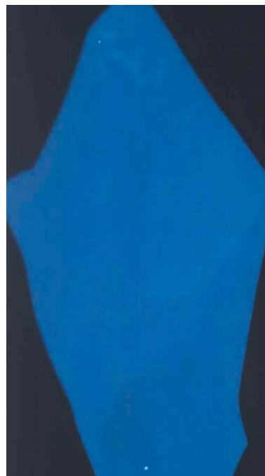
Fig. 13 Piece of a siloxene-filled alumina membrane under UV irradiation. 6
